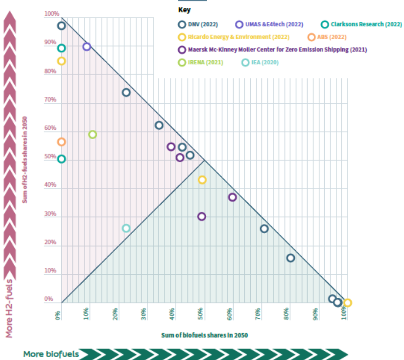
Figure 1: Mapping most recent fuel mix scenarios: Hydrogen (H2)-fuels scenarios versus Biofuels scenarios.
